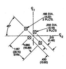
**18.** Hole pattern no. 436 accommodates t0-3s (4-pin). Available in UP, UP1, UP2, HP1, and HP3 series heat dissipators.
