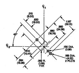
28. Hole pattern no. 64 (Universal) accommodates T0-3s, D0-4s, T0-15s, T0-6s, T0-36s, or other stud mounted devices up to ¼" diameter. Available in UP, UP1, UP2, HP1, and HP3 series heat dissipators.
