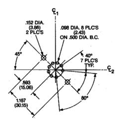
**19.** Hole pattern no. 2 accommodates T0-6s or T0-36s. Available in UP, UP1, UP2, HP1, and HP3 series heat dissipators.
