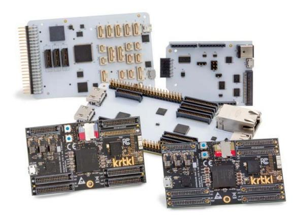
Each baseboard has its own on-board memory/identification chip that tells your snickerdoodle what's plugged in and automatically loads the right package to get all your peripherals working without you lifting a finger.
