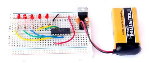
snapVCC eliminates this additional circuit by putting the regulator right on top of the 9V battery.
