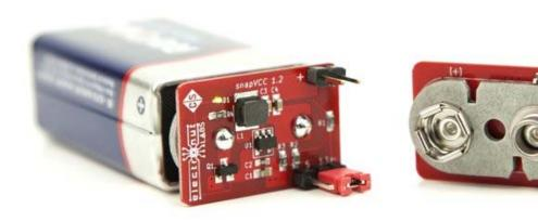
snapVCC is a highly portable and convenient power supply for your electronics projects. It's designed to fit right on a 9V battery and give you 3.3V or 5V power wherever you need it.
