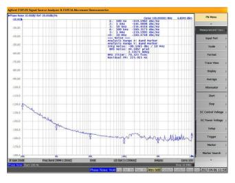
ERASynth rev2 phase noise at 1 GHz RF output.
