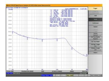
ERASynth rev2 phase noise at 10 GHz RF output.
