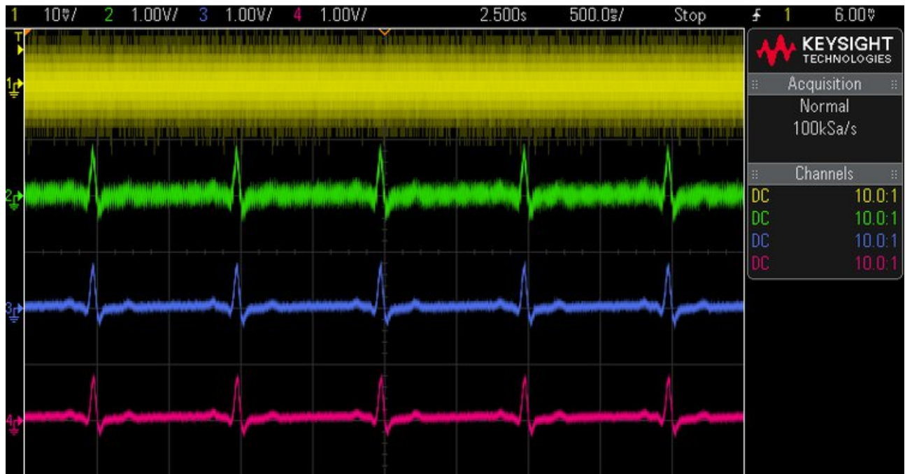
ECG signal through various stages of the AFE module. Yellow trace is the input and pink trace is the output.
