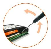
To turn on a switch, use a tool such as a small screwdriver to gently push the switch forward
