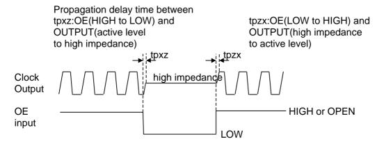
NOTE: A disable clock output does not synchronize with OE, because internal quartz oscillator is continuous.
