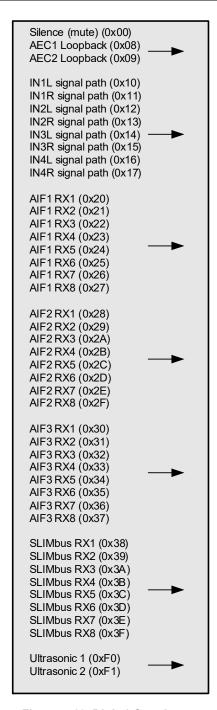
Figure 4-16. Digital-Core Inputs
