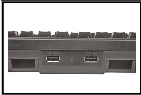
Down Stream ports
