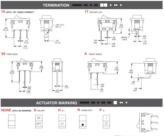
NOTE: Orientation of actuator marking and terminals.
