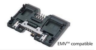
The CCM02 MK II connectors with landing contacts are dedicated for applications where the reader usage is high and the life span of the card is a key consideration. A connector with contacts which land on the card, rather than slide over it, should be specified so as to minimize card wear. The CCM02 has been redesigned to give an even higher performance in a compact, affordable package.
