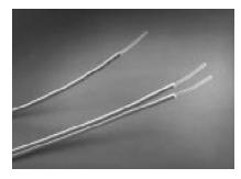
When using the duplex connector arrangement, the separated duplex cable should be stripped to roughly equal lengths on each cable end.
