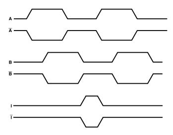
Waveforms for Encoders with Line Drivers.
