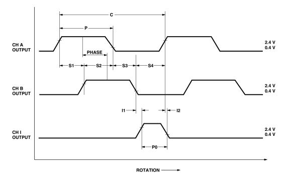
Waveforms for Encoders without Line Drivers.
