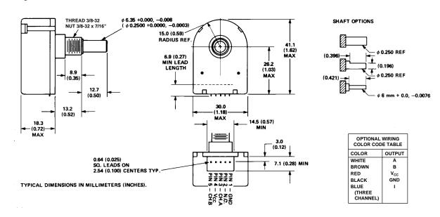
\*Note: For the HEDS-5700, Pin #2 is a No Connect. For the HEDS-5740, Pin #2 is Channel I, the index output. The HEDS-5700 is quickly and easily mounted to a front panel using the threaded bushing, or it can be directly coupled to a motor shaft (or gear train) for position sensing applications.
