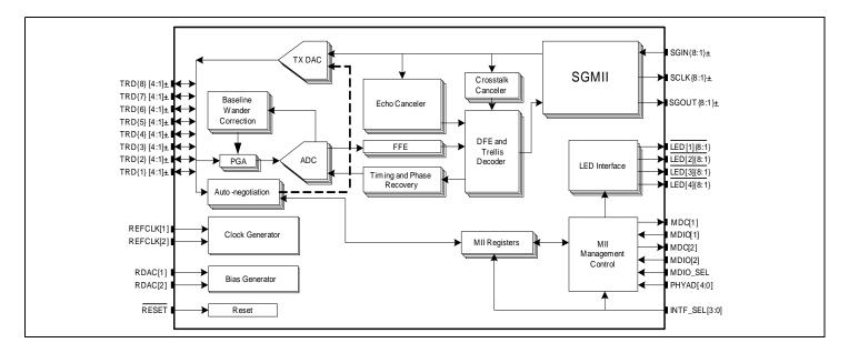
The BCM5488 consists of eight complete 10/100/1000BASE-T Gigabit Ethernet transceivers integrated on a single monolithic CMOS chip. The BCM5488 is optimized for low power and small footprint size to enable high-port density applications. By lowering system cost and reducing power dissipation by nearly 30 percent, the BCM5488 enables a new class of cost-effective Gigabit Ethernet equipment, driving the delivery of Gigabit Ethernet bandwidth to the desktop.
