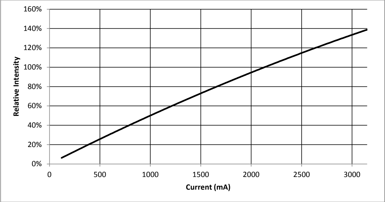
Figure 3: Typical Flux vs. Drive Current, Tj = 25°C
