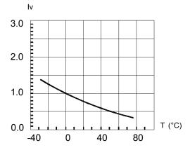
Fig. 6 Relative Luminous Intensity vs. Temperature
