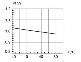
Fig. 5 Forward Voltage vs. Temperature
