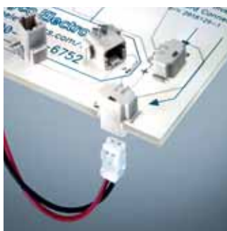
This Tyco Electronics™ SMT thru-board connector provides a way to bring power from the underside of a Thermal Clad IMS board, eliminating issues of dressing wires on the top side of LED boards.
