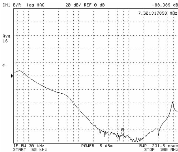
Figure 3 - Common Mode attenuation, 0.05-100 MHz. Source and load resistances are 50 \Omega . Two 0.1 \mu F Y-caps to common line. Vertical scale: 20 dB/div, with zero dB level marked by arrow.
