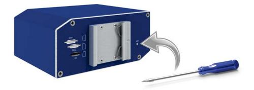
Figure 39: Router reset
