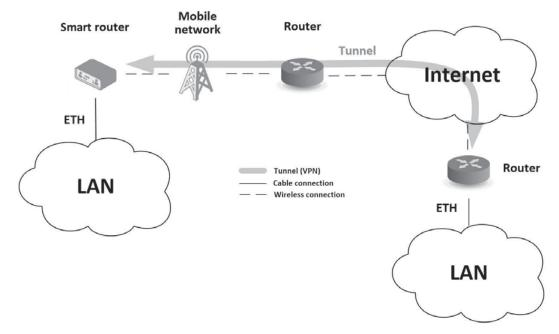
Figure 3: Using a VPN tunnel
