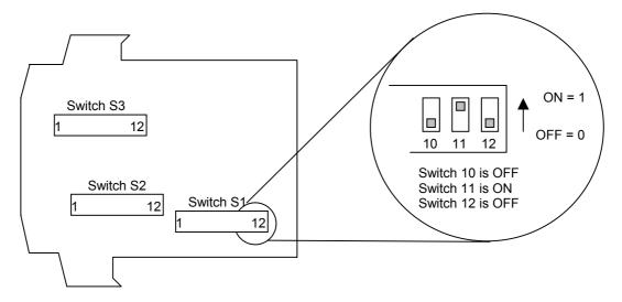
Switch S1 and S2 configure the input type and range, and switch S3 configures the output type, range and a few additional functions. The switch settings are explained in the next few pages. The diagrams refer to switch positions 0 and 1, with 0 being OFF and 1 being ON. This is illustrated in the picture above.
