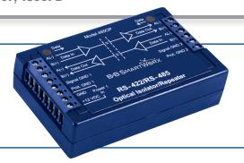
Model 4850P is an optically isolated RS-422/485 signal repeater. In addition to 2KV isolation on the data lines, it can be used to extend RS-422/485 circuits an additional 1.2 km (4,000 ft.), thereby doubling the range. An added benefit is the ability to add another 32 nodes to an RS-485 network and join 2 and 4 wire systems.
