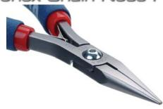
Features very fine tips, "eased" edges of the inner jaw to reduce the risk of damage to the workpiece during forming, and a long jaw for extended gripping power. Available with smooth or serrated jaws. Standard & Short Chain nose pliers have tips dimension of 1.2mm W x 1.4mm H (.050" x .060").
