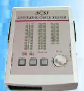
This SCSI tester can test cable with up to 68 lines. With the optional PC or MAC cable Test Unit it can be upgraded to a multi cable tester. The transmitted and received data between the two ends of the cable will be compared. The result is shown by LEDs.
