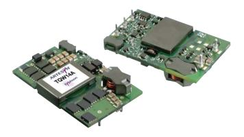
This series is a Quarter-Brick, wide-input intermediate bus converter (IBC). Capable of operating from any input voltage in the range 36 Vdc to 75 Vdc, this high efficiency isolated dc-dc converter module generates a semi-regulated 12 V output and can deliver up to 14 A. This series features a low profile open-frame construction and has an industry standard quarter-brick footprint.
