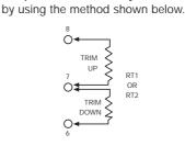
**EXTERNAL OUTPUT TRIMMING** Output can be externally trimmed
