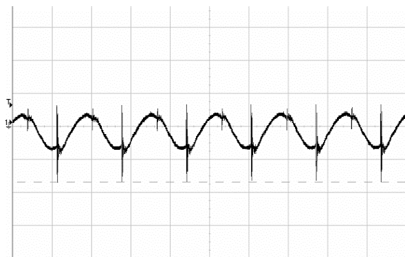
Figure 3 Output ripple & noise (2μs/div, 20mV/div), see Figure 15 for test configuration
