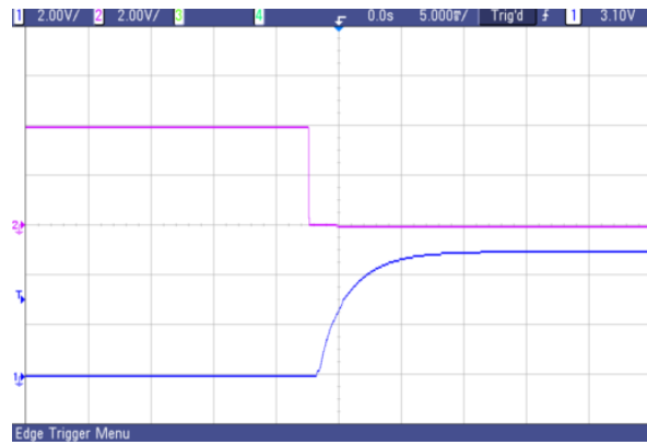
Fig. 68 AVO75-48S05 typical start-up from CNT on
