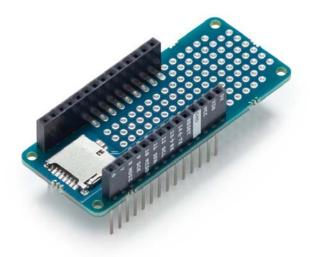
The Arduino MKR SD Proto Shield allows you to easily connect an SD card to your MKR form factor board. Use it to enhance the IoT features of your MKR1000, as well as store data coming from the web or sensors read by your board!
