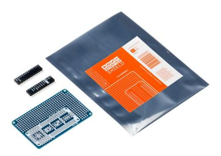
Need more room for your MKR Proto Shield? The MKR Proto Large Shield fits onto your MKR board using its provided female/male headers, and enables you to fix it wherever you want with the mounting holes. This shield features a larger prototyping area with more than 300 solder points and makes connecting components to your board super simple, thanks to the silk that indicates the MKR board pins location.
