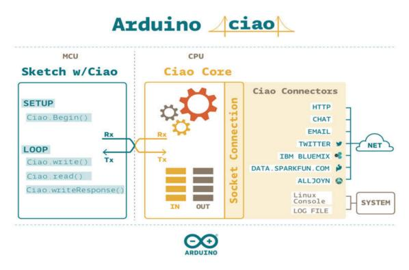
Arduino Ciao is an easy-to-use and powerful technology that enables Arduino sketches to communicate intuitively with the "outside World". It aims to simplify interaction between microcontroller and Linino OS, allowing a variety of connections with most common protocols, third-party services and social networks.
