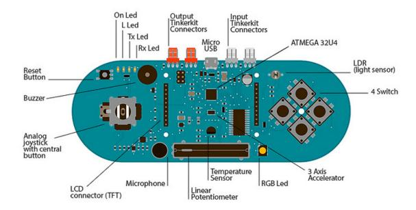
The design of the Esplora board recalls traditional gamepad design with an analog joystick on the left and four pushbuttons on the right.
