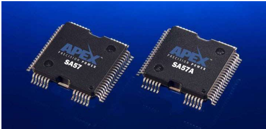
FIGURE 2. 64-PIN QFP, PACKAGE STYLE HQ
