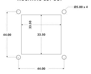
The joystick is mounted from beneath the panel, with the bezel fitted onto the front face of the panel. It is recommended to use No. 2 self tapping, pan head screws, the length of which must be determined subject to the thickness of the panel.
