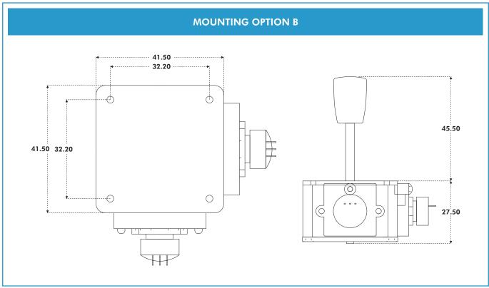
Note: The dimensions shown are for a generic two axes 5000 Series with the F type handle. For specific dimensions of this or any other configuration please refer to Apem.
