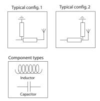
The matching network has to be individually designed using one, two or three components.
