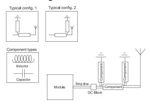
The matching network has to be individually designed using one, two or three components.
