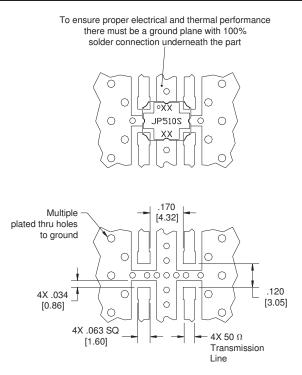
Dimensions are in Inches [Millimeters] JP510S Mounting Footprint
