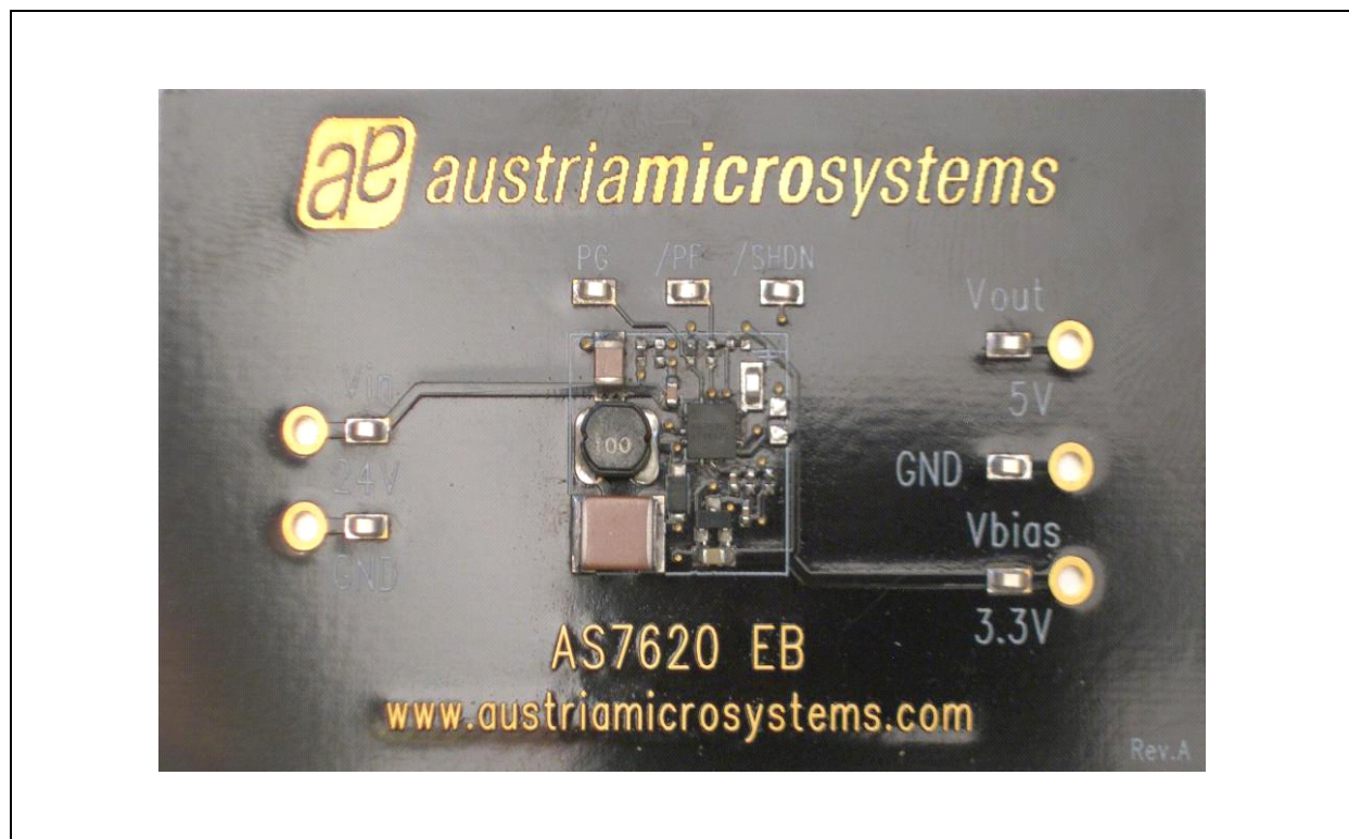
Figure 1. Demo Board Photograph
