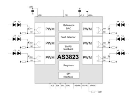
The AS3823 is a 6 channels precision LED controller for use in LCD backlight panels. Dynamic power feedback controls the external power supply to guarantee best efficiency. Build in safety features include thermal shutdown as well as open and short LED detection. The device is programmable via serial interface.
