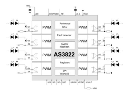
The AS3822 is a 8 channels precision LED controller for use in LCDbacklight panels. Dynamic power feedback controls the external power supply to guarantee best efficiency. Build in safety features include thermal shutdown as well as open and short LED detection. The device is programmable via serial interface.
