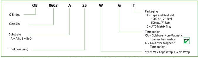
The above part number refers to a Q-Bridge, (EIA case size 0603), Aluminum Nitride (AIN) substrate, Thickness 25 mils., Style W, G Termination (Gold over Magnetic Termination), with Tape and Reel Packaging.
