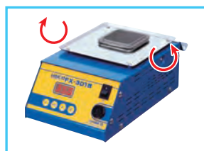
Loosen the screw on both sides.
