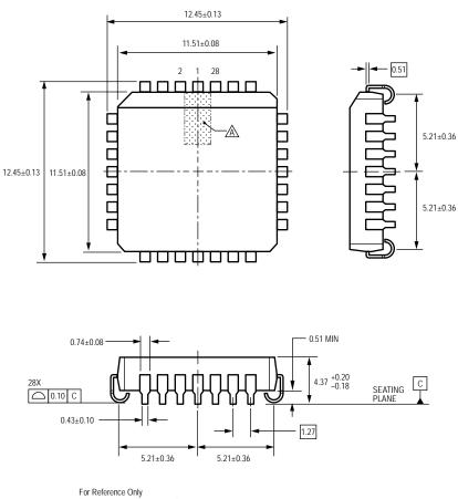
For Reference Only (reference JEDEC MS-018 AB) Dimensions in millimeters Dimensions exclusive of mold flash, gate burrs, and dambar protrusions Exact case and lead configuration at supplier discretion within limits shown Terminal #1 mark area
