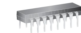
16-pin DIP (A package)
