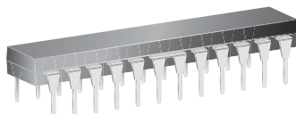
Package B, 24-pin DIP with exposed tabs
