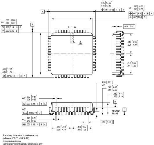
Dimensional minimum in brackets, for reference only Dimensions exclusive of mold flash, gate burs, and dambar protrusions Exact case and lead configuration at supplier discretion within limits shown
