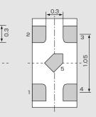
Pin 5 is short to pin 3 inside the package.
