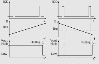
Operating Point Timing Release Point Timing
