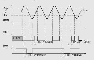
Note1) In power down mode, Output is kept current status. Note2) When VDD is supplied ,output settling time after power supply voltage exceeds 1.6V is equal to TPD2.
