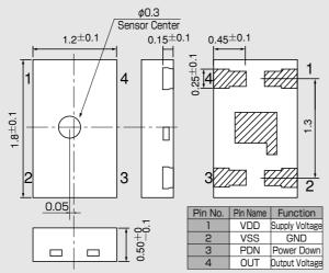
Note1) The sensor center is located within the  $\phi$ 0.3mm circle.
