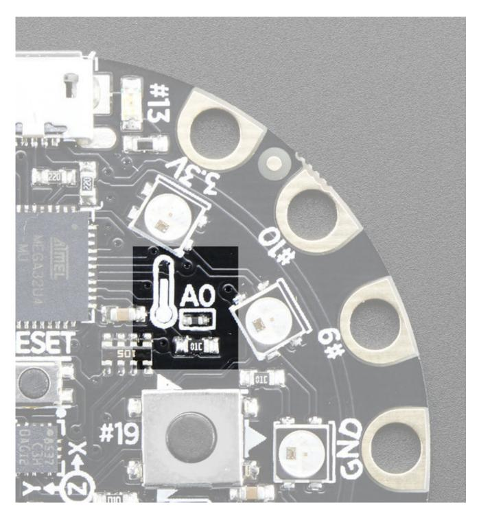
There is an NTC thermistor (<u>Murata NCP15XH103F03RC</u>) that we use for temperature sensing. While it isn't an all-in-one temperature sensor, with linear output, it's easy to calculate the temperature based on the analog voltage on analog pin **#A0**. There's a 10K resistor connected to it as a pull down.
