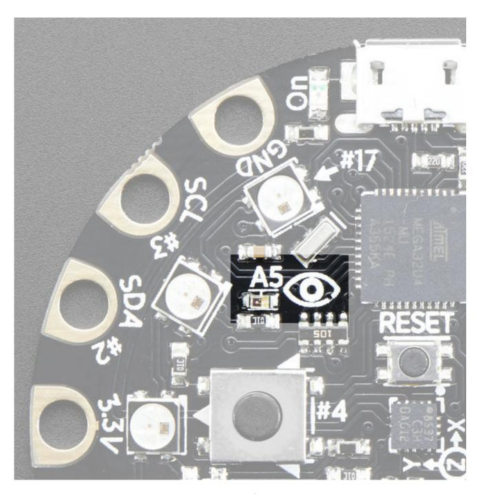
There is an analog light sensor, <u>part number ALS-PT19</u>, in the top left part of the board. This can be used to detect ambient light, with similar spectral response to the human eye.
