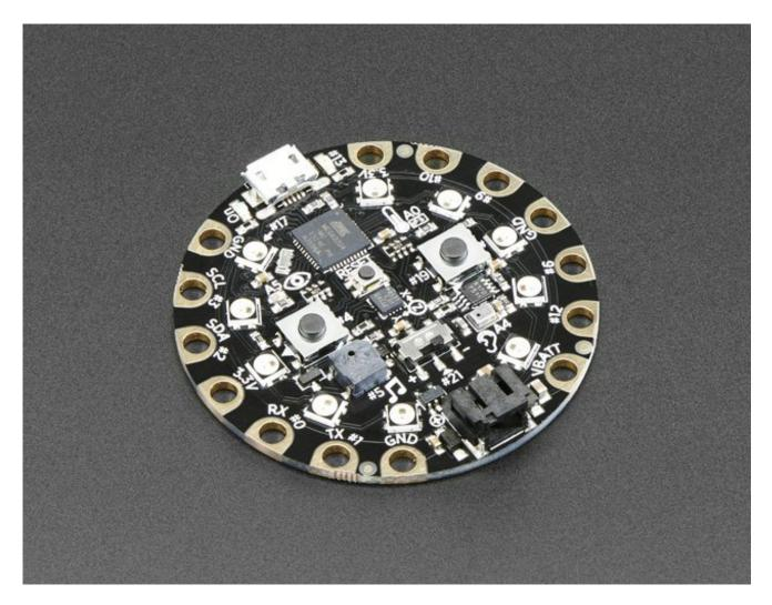
Circuit Playground has built-in USB support. Built in USB means you plug it in to program it, it just shows up - all you need is a Micro-B USB cable, no additional purchases are needed! With the new 1.6.4+ Arduino IDE, it takes only a few seconds to add support (http://adafru.it/nb4). The Circuit Playground has USB HID support, so it can act like a mouse or keyboard to attach directly to computers.
