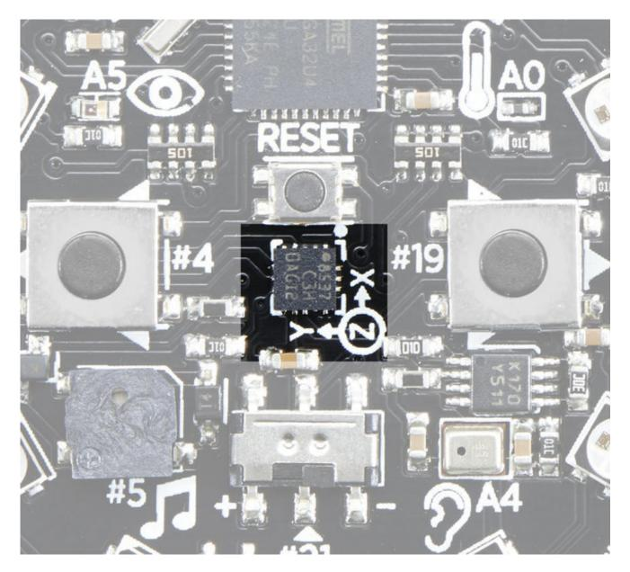
A LIS3DH 3-axis XYZ accelerometer is in the dead center of the board and you can use it to detect tilt, gravity, motion, as well as 'tap' and 'double tap' strikes on the board. The LIS3DH is connected to the hardware SPI pins (to leave the I2C pins free) and has the CS pin on digital pin #8 and an optional interrupt output on digital pin #7 (also known as IRQ #4)
