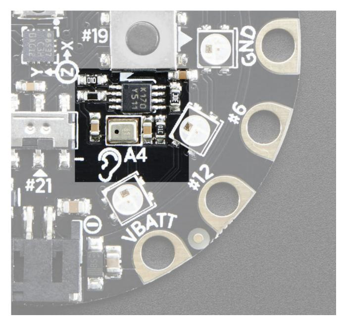
A MEMS microphone can be used to detect audio levels and even perform basic FFT functions. You can read the analog voltage corresponding to the audio on analog pin #A4. Note that this is the raw analog audio waveform! When it's silent there will be a reading of ~330 and when loud the audio will read between 0 and 800 or so. Averaging and smoothing must be done to convert this to sound-pressure-level.
