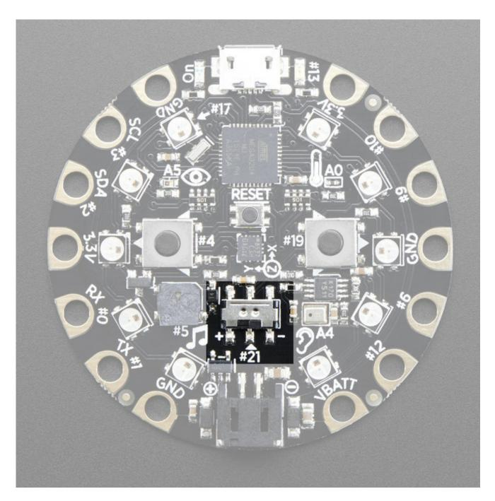
There is a single slide switch near the center of the Circuit Playground. It is connected to digital **#21** and will read LOW when slid to the left, and HIGH when in the right hand position
