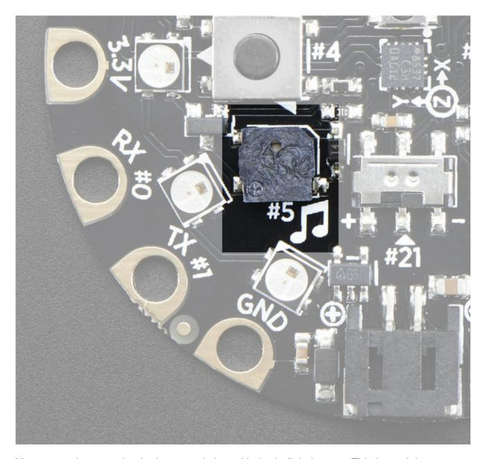
You can make your circuit playground sing with the built in buzzer. This is a miniature magnetic speaker connected to digital pin **#5** with a transistor driver. You can use PWM at varying frequencies to make basic tones.
