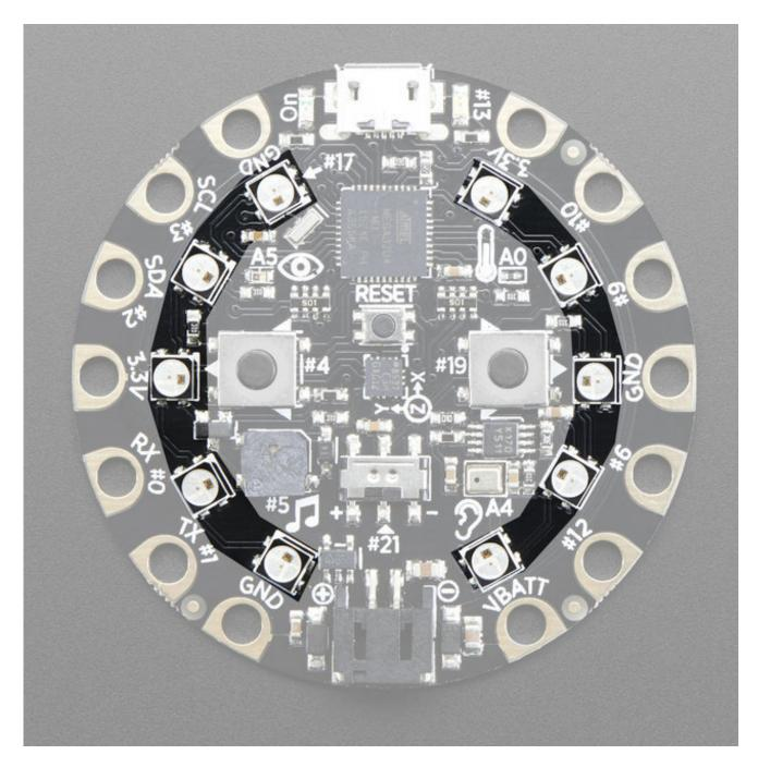
Each Circuit Playground comes with 10 'NeoPixels' (technically, SK6812-3535 chips). These are connected to digital pin **#17** and are powered by the 3.3V regulator. This is technically undervolting but we test them at this voltage and they work fine, if slightly tinted
