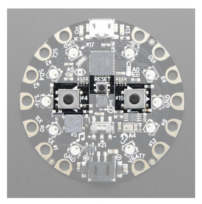
There are three tactile pushbutton switches. One is the Reset button. Press this button once to reset, double-click to enter the bootloader manually.
