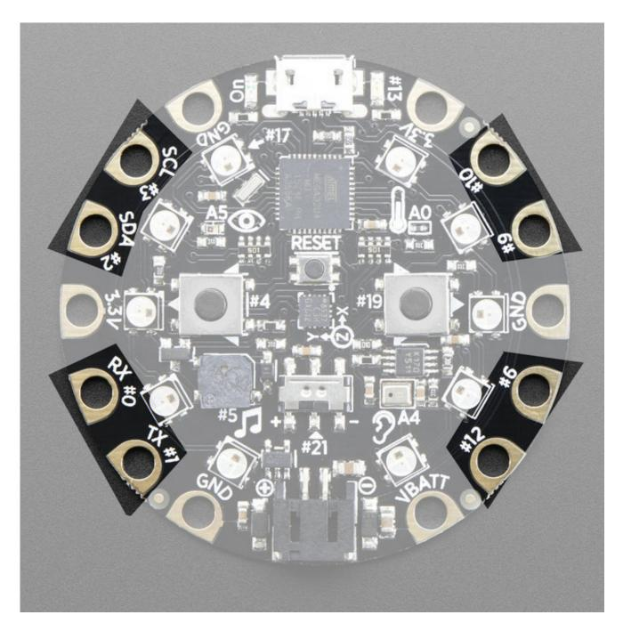
All 8 non-power pads around the circuit playground have the ability to act as capacitive touch pads. Each pad has a 1Mohm resistor between it and digital pin #30. You can toggle this pin to control whether the resistor is a pullup or pulldown or floating. Note that this means that all the pads have a 2Mohm resistance between them.
